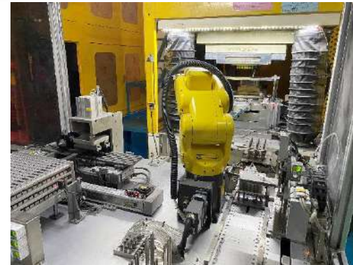
Multiple cavities molding machine with robot arm
