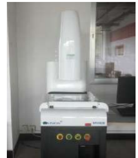
Automatic image measuring instrument Automatic zoom lens 0.7~4.5X90mm working sight distance 0.0005mm resolution ratio
