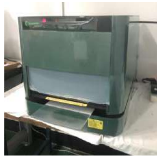
Desktop X-ray fluorescence coating thickness gauge Detectable element range: No.13 aluminum-No.12 Uranium 10 element can be analyzed in each layer
