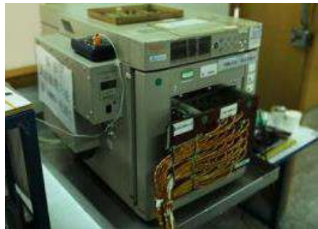
Self-developed test chamber integrated of mutli test equipment Lowest temperature reaches -60 ^{\circ} C Labview development control program achieves automatic data collection
