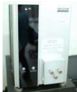
Korean SEC electronic Microscope 60,000x MAX
