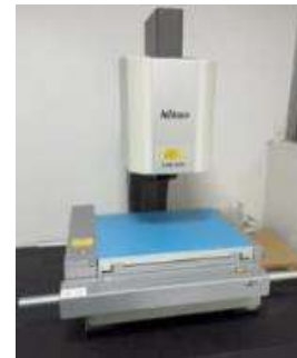
Nikon 2.5D projector Max resolution reaches 0.1 \mu m
