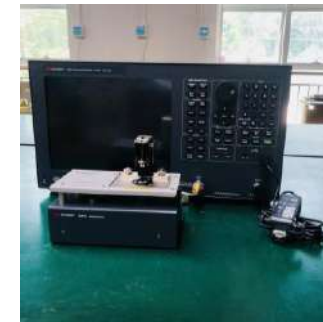
Vector Network Analyzer Support frequency 5Hz~3 GHz/50 or Transfer/reflect or parameter S test
